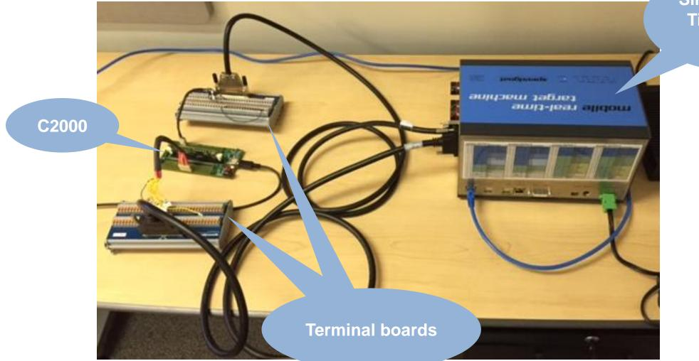
Simulink Real Time Target Machine
