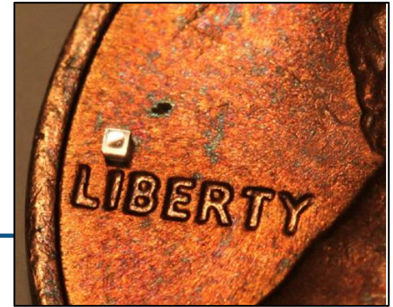
Microtech's submillimeter sensor, dotting the "I" on a U.S. penny.
