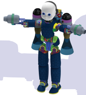
Redesign of the iCub humanoid robot with jetpack.
