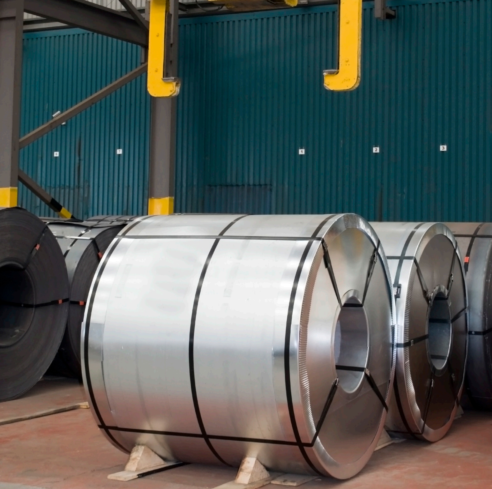
Cold-rolled steel coils. Ruukki Metals processes 60,000 coils annually. To ensure quality, engineers use a MATLAB application to aggregate and analyze up to 4000 different measurements for each coil.
