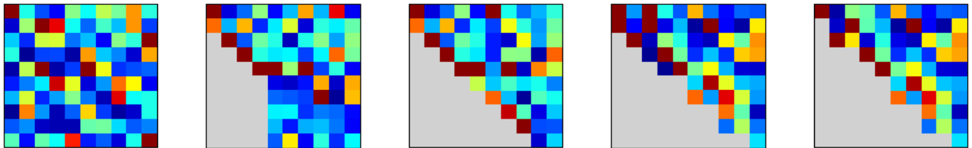
FIGURE 2. Eigenvalues of a nonsymmetric matrix. Left to right: The input—a random 10-by-10 matrix; halfway through the orthogonal reduction to Hessenberg form; Hessenberg form, upper triangular plus one subdiagonal; partway through the nonsymmetric QR iteration; and the final real Schur form with real eigenvalues and 2-by-2 blocks with complex pairs of eigenvalues on the diagonal.
