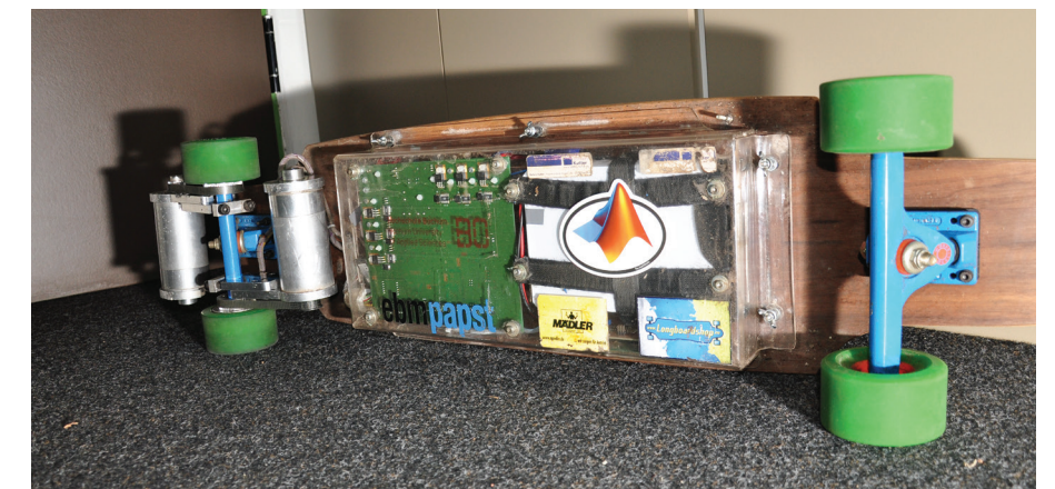
FIGURE 1. The underside of the e-longboard showing two BLDC motors on the left.
