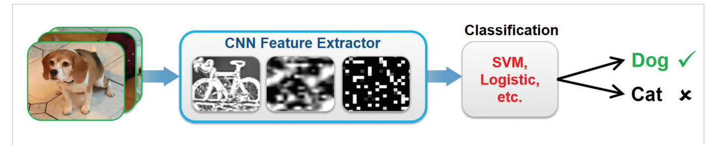
FIGURE 1. Workflow for using a pre-trained CNN to extract features for a new task.
