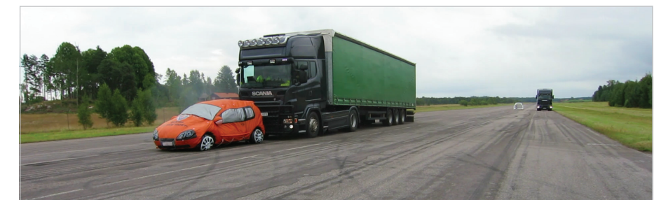
FIGURE 1B. A typical AEBS scenario: truck with AEBS installed approaching a slow-moving vehicle.
