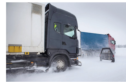
FIGURE 4. A controlled road test of the AEBS software. The trapezoidal object between the two vehicles is a “soft target,” designed to resemble a vehicle, that is used to “fool” the radar and the camera.
