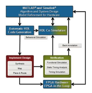
Figure 1. Integrated workflow from system design to hardware with MATLAB and Simulink.
