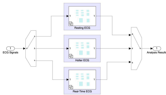
ECG signal analysis algorithms modeled in Simulink.
